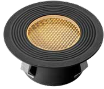
Onyx 90 RA (245D) Aluminium - Anthracite LED 2 W 2.700 K 76 lm 78 x 105 mm (H x Ø) Trou de forage 90 mm
